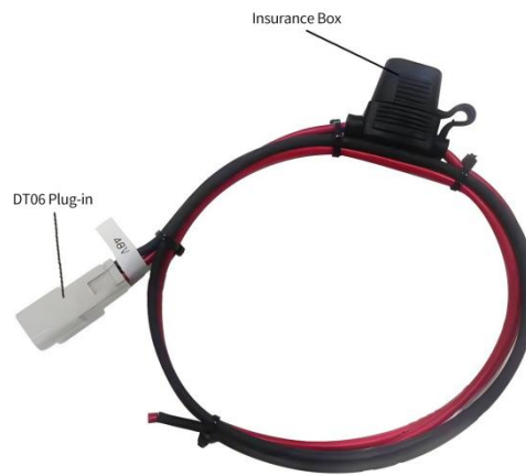
Figure 4-4 Customer power harness
